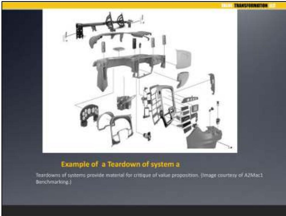
Here is an example of the documentation of a static breakdown. In this case the product was disassembled and the parts handled and assessed culminating in this graphic.
